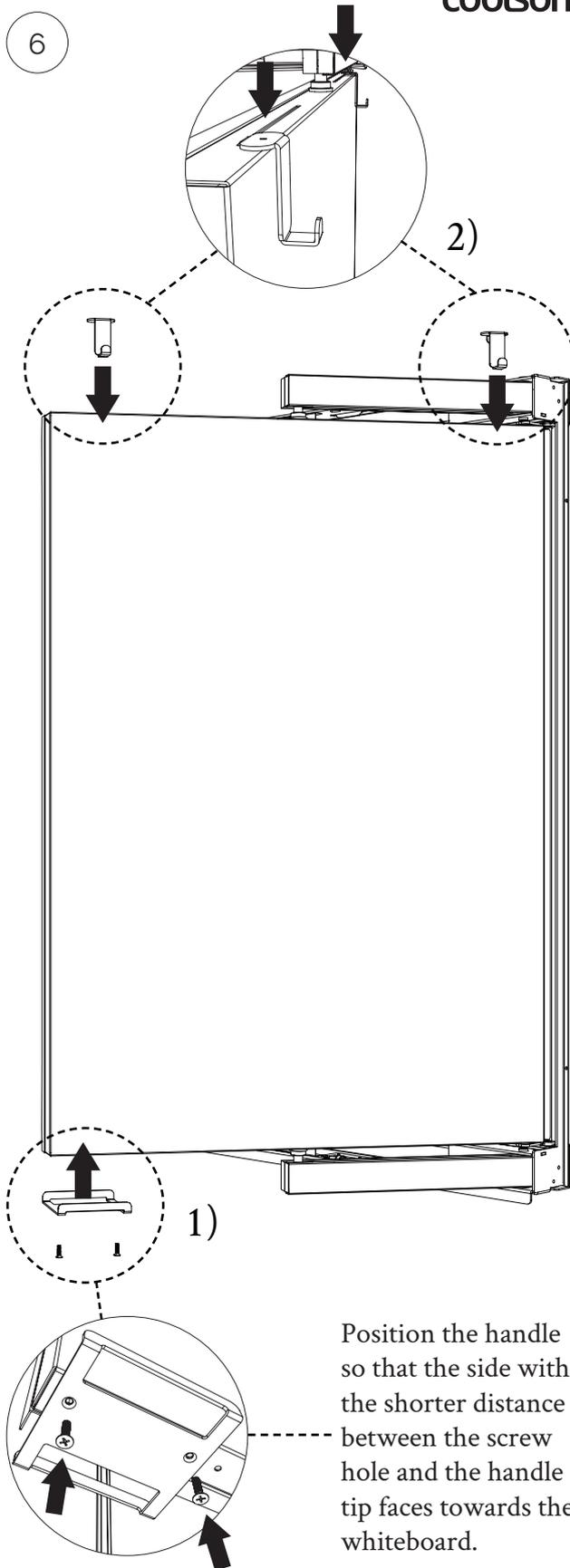
1) Open the door and attach the handle with two countersunk M4 screws.
