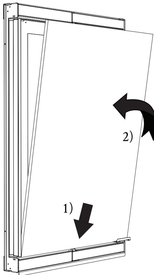
Attach the acoustic board. The acoustic board is held in place with magnets. Install the board to the side containing the acoustic board framing by 1) first sliding its bottom edge onto the door's flanged edge. 2) Then, push the top edge of the acoustic board into the frame.
