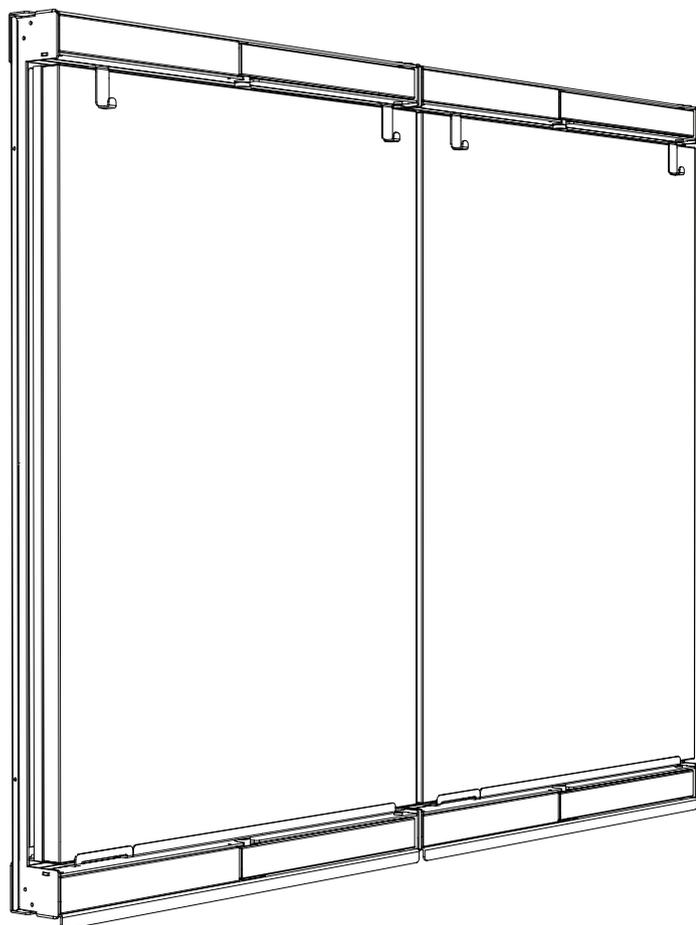
In case you are installing several Flipmodes side by side, we recommend to use the side edge of the first Flipmode for installing the next one in the correct position, and so forth.
