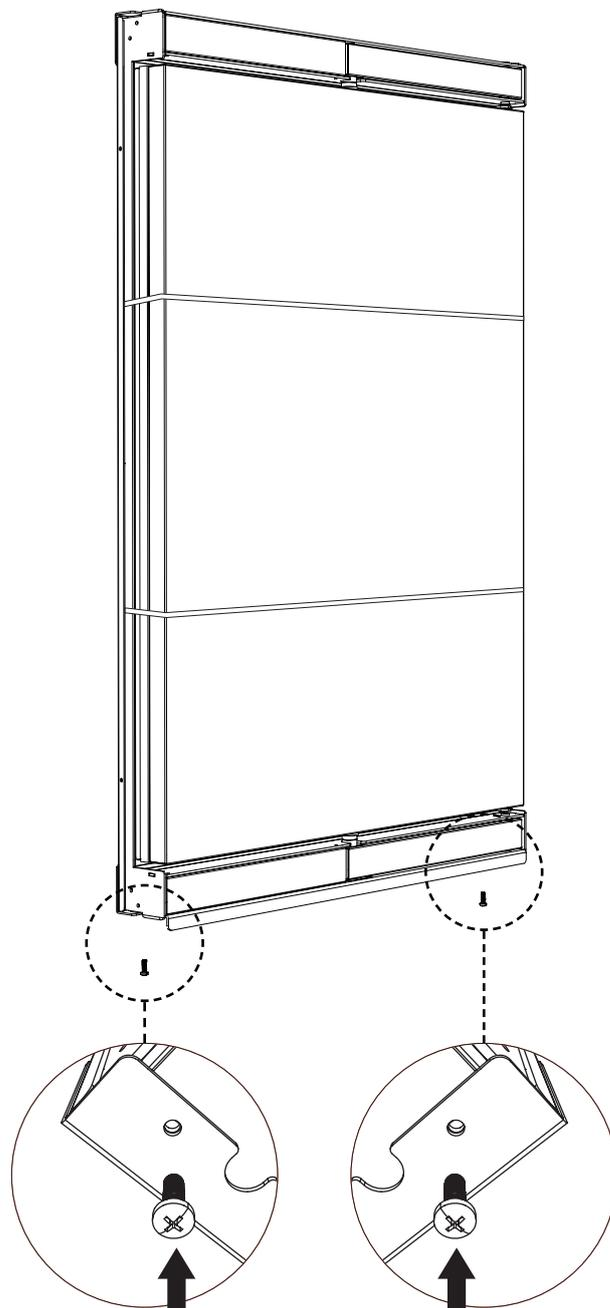
Secure the frame to the wall mount by attaching it with the included M5 pan head screws.
