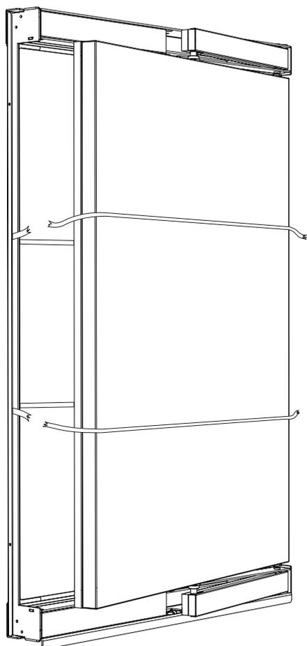
The straps should be cut on both sides, and once that is done, they can be removed by pulling them out through the slits on the sides.
