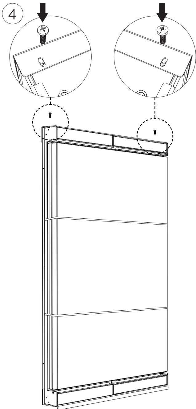
Next, install and secure two M5 pan head screws on the top of the frame while pushing the top of the Flipmode frame towards the wall.
