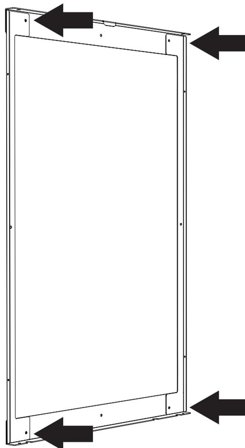
Install the wall mount to the wall by using a screw in each corner. Please make sure to use heavy-duty wall anchors. The mounting holes are designed for 6 mm metric screws, which enables the use of alternatively 3/16 inch or 1/4 inch screws.
