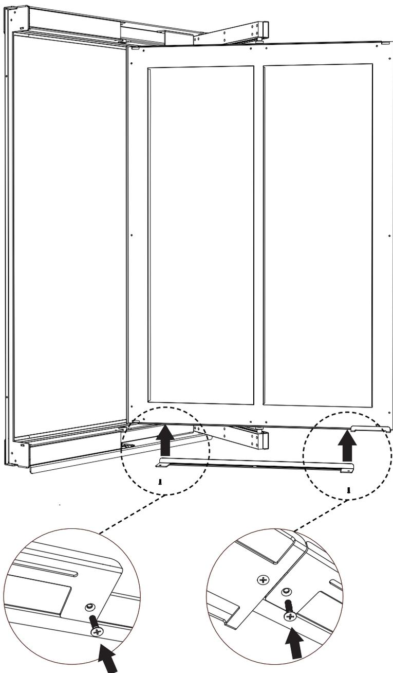
Install the marker tray with two countersunk M4 screws. In order to do this, first fully open the door and slightly close it by turning outwards the side with the framing for the acoustic board (seen in the picture above). This way it will be easier to attach the screws to their corresponding holes. Make sure that the folded side of the marker tray is positioned towards the whiteboard.
