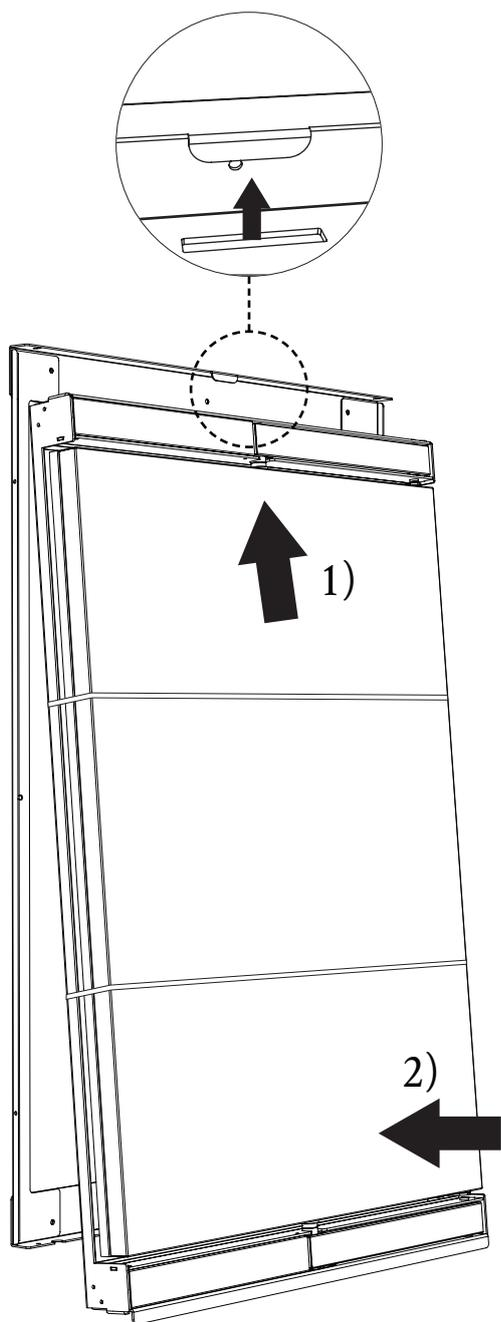
Place the Flipmode frame in the secured wall mount by...
